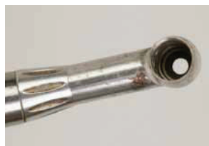
Figure 9. Corrosive effects of sterilization
