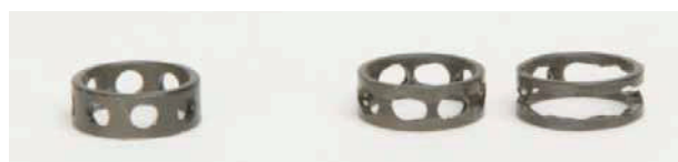
Figure 14. Bearing retainer showing stages of degradation
