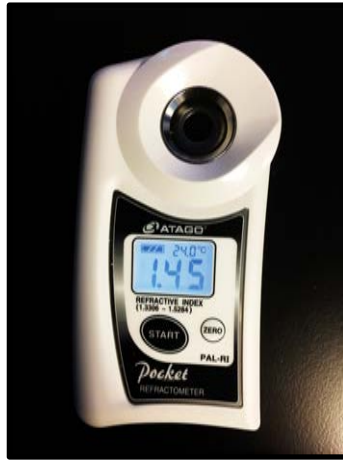
Figure 10. Refractometer used for determination of the Refractive Index (RI) of the cleared tissue, verifying that the RI of the 63% TDE solution before imaging in the light sheet microscope is 1.45.
